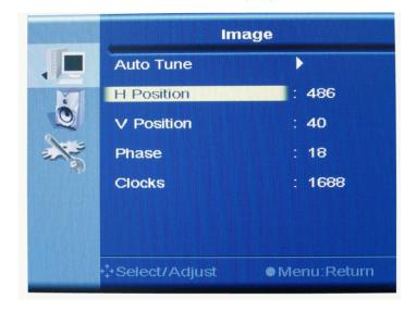
b. Press "△" or "▽" to adjust the horizontal position. Then press "1" to confirm the adjustment and back to Image menu.
